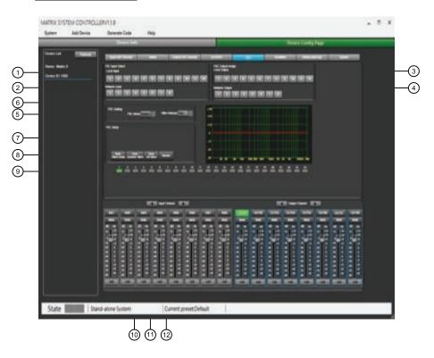
**FBC** or **Feedback Canceller** is a function which eliminates feedback automatically. Feedback occurs unexpectedly in a system where there are microphones and speakers nearby one of the other. This loop effect is an electro-acoustic resonance which generates an unpleasant frequency noise.
