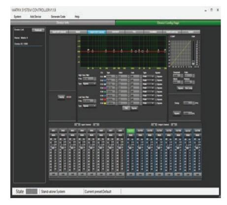
Same menu as the Input DSP Channel, without the Expander/Gate section. The Parametric EQ features 8 bands here, instead of 5 bands for the Inputs. Please refer to page 13.
