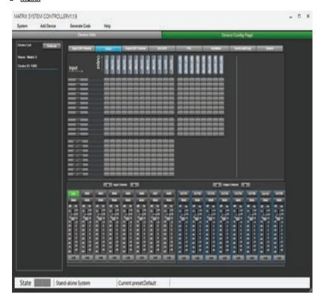
This part of the software is used to route inputs to outputs through a graphical representation as a matrix. By clicking on the gray boxes several inputs can be assigned to several outputs. If the connection is active the box turns green, otherwise it remains gray.
