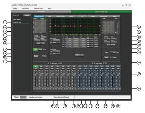
The **Input DSP Channel** is the first page appearing when the Editor Software is opened.
